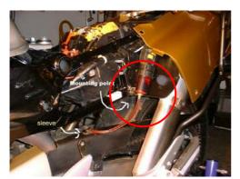
The RMV can be mounted inside the left hand rear fairing, as shown on the left. The more vertical the RMV the better and remember to avoid exhaust and engine components.
